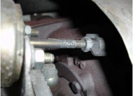
Once you have wound the adjuster up to the mark you had made on the actuator rod (approx 5mm), tighten the locknut back against the collar to prevent it from moving.
