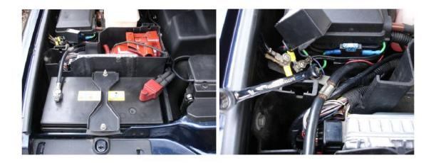
Remove the Plastic Battery/ECU cover, and undo the Battery lead to chassis Earth retaining nut with a 10mm Spanner.
