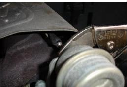
You need to turn the knurled adjuster on the actuator, in order to make your adjustment. However, it can be quite stiff so to prevent damage to the diaphragm inside the wastegate actuator, clamp the actuator rod in place with some mole grips. If the knurled adjuster is tight, use some pliers to turn it. You could use a squirt of wd40 as well, but be prepared for some smoking when it all gets hot!!!
