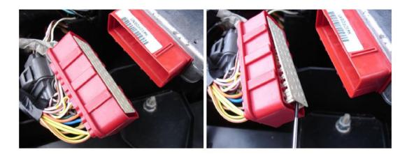
Take the Red ECU plug off it's socket. There is a retaining clip on the other side of the plug, which you will need to press down to release it. Using a small screwdriver, gently prise off the white plastic cover, to expose the terminals.
