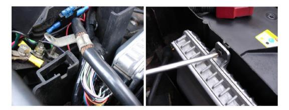
Now lift the Battery Earth cable off the chassis earth post, then undo the engine ECU retaining screw.
