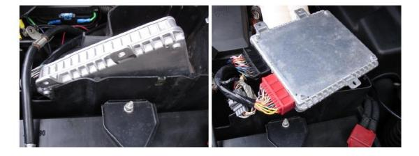
Tilt the ECU up and lift out. Rest the ECU, upside down on top of it's housing.
