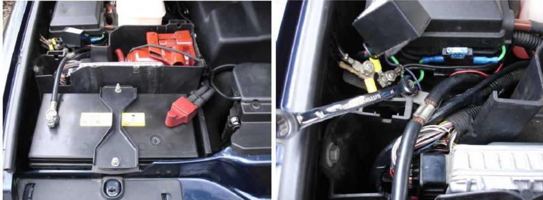
Remove the Plastic Battery/ECU cover, and undo the Battery lead to chassis Earth retaining nut with a 10mm Spanner.
