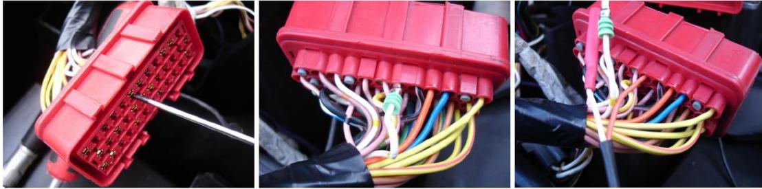
Now we are confident we have the right wire, using a very small screwdriver, or a pin, release the connector from the plug by prising gently on the small retainer (Left). Once the connector has been released, pull it right out of its hole (Middle). Now put the (White) Female type connector from the TD5 BOOSTER into this hole. Push it right in and you should hear or feel a click as it locates. Give it a gentle tug, and it should stay put (Right).
