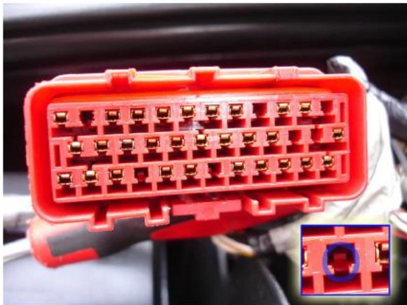
Once you've removed the plastic cover, you'll see all of the connectors in the plug. Each of these connectors are held in place with a small plastic retainer. Looking at the inset picture (connector removed for clarity) you'll see the retainer quite clearly.
