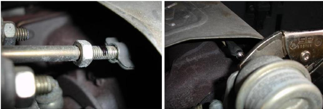
You need to turn the knurled adjuster on the actuator, in order to make your adjustment. However, it can be quite stiff so to prevent damage to the diaphragm inside the wastegate actuator, clamp the actuator rod in place with some mole grips. If the knurled adjuster is tight, use some pliers to turn it. You could use a squirt of wd40 as well, but be prepared for some smoking when it all gets hot!!!
